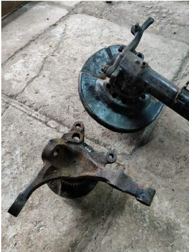
Images: Nissan sourced hub (Left) vs. Original Datsun Hub (Right)
