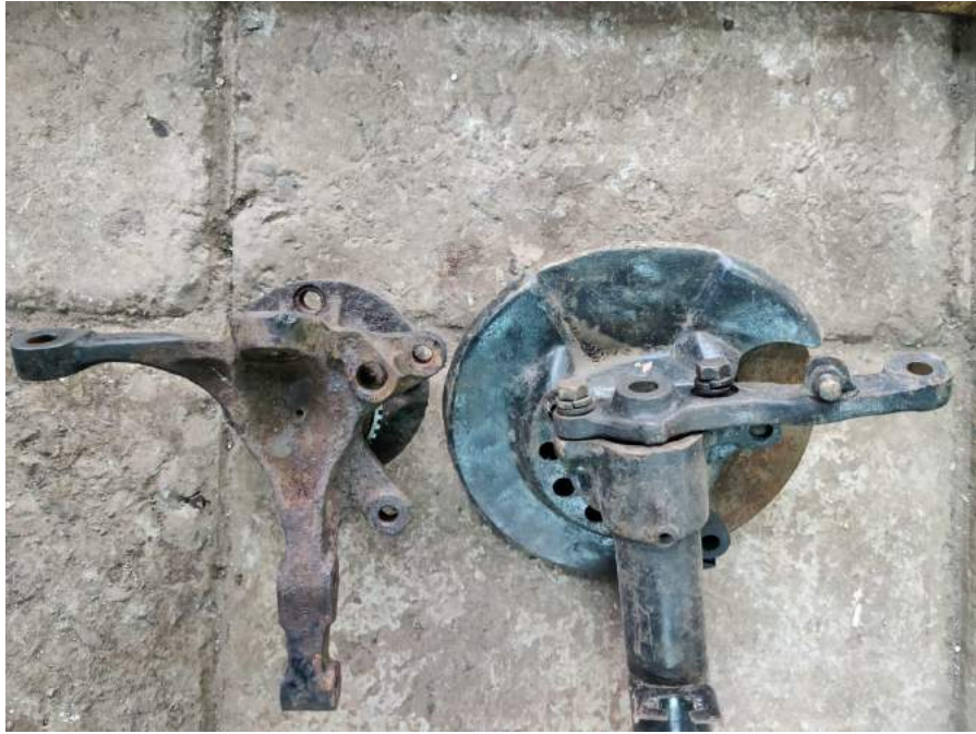
Images: Nissan sourced hub (Left) vs. Original Datsun Hub (Right)
